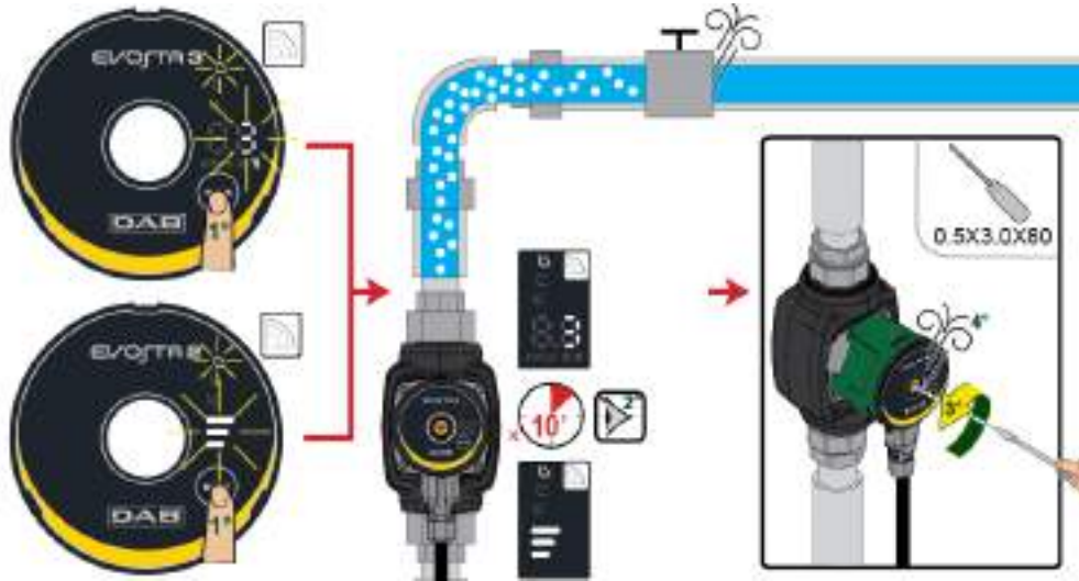
Figure 8: Venting of the pump
