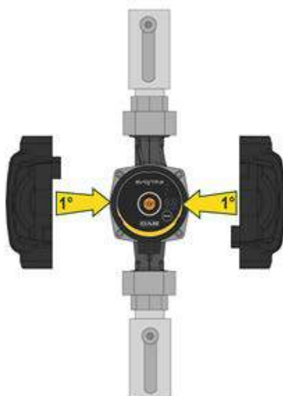
Figure 7: Insulating the pump body
